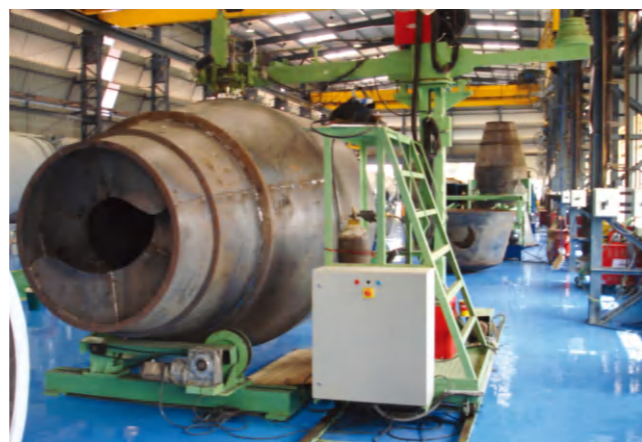
水泥罐焊机 Custom built welding manipulator
