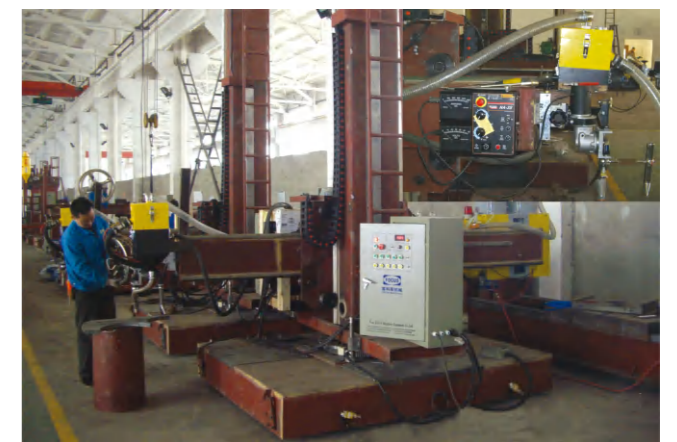
焊接中心 Welding manipulator with DC1000
