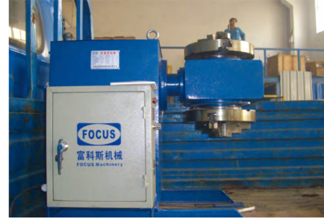
双卡盘管子变位机 Welding positioner with chuck
