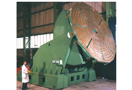
120吨特制变位机 WP120 custom built positioner
