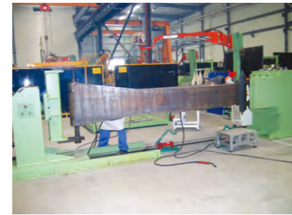
头尾式单回转变位机 Head and tail stocks and single turning positioner
