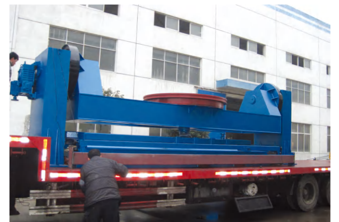
双座变位机 Cradle welding positioner
