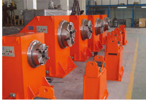
头尾式变位机 Welding positioner with chuck
